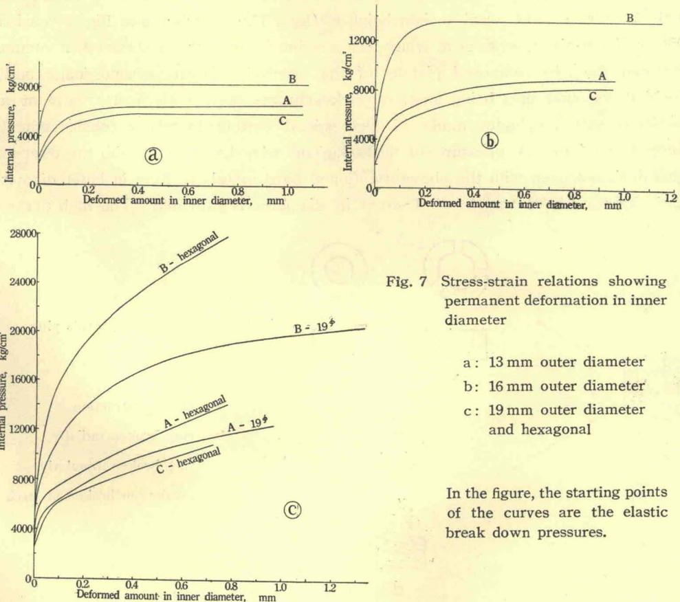
Fig. 7 Stress-strain relations showing permanent deformation in inner diameter
