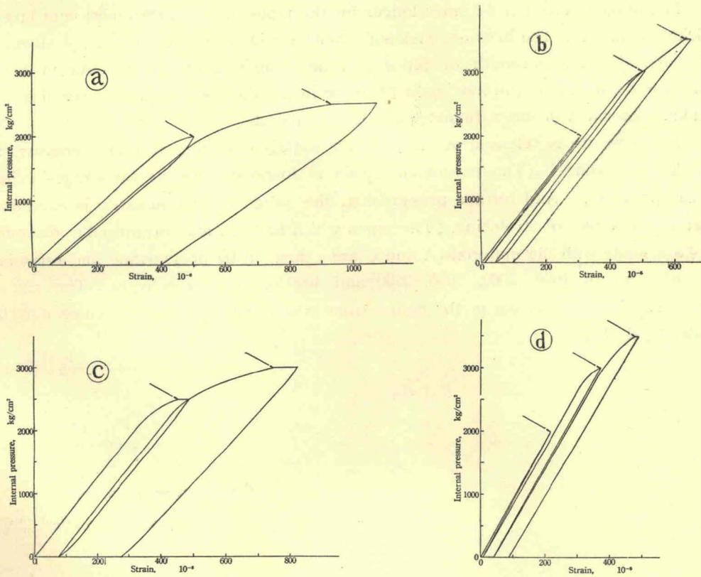
Fig. 5 Stress-strain relations showing linearity and flow
